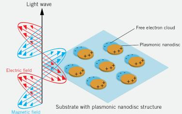
Nanoplasmonic sensing is an optical technology for detecting and monitoring material and interface processes under in situ conditions.
