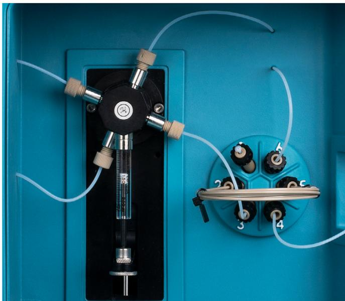
The Insplorion S2 comes equipped with state of the art syringe pump as well as an automatic injection valve. This allows for precise handling of the sample and buffers and remote control, using the Insplorion InControl software. Syringes and sample loops with different volumes are available.
