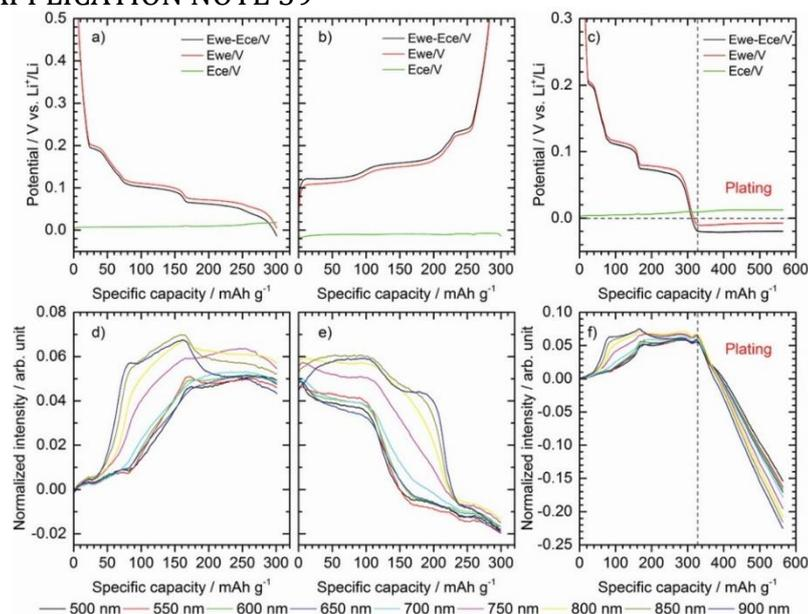
**Figure 2:** Potential profile of lithiation and delithiation of graphite (WE) and Li (CE) half-cell are presented in (a) and (b), respectively. The corresponding intensity of the optical signal is shown in (d) and (e). The zoomed-in figures (c) and (d) present the Li plating region.
