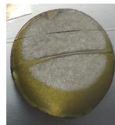
**Figure 3:** Post-mortem image of the graphite electrode that was over-lithiated.
