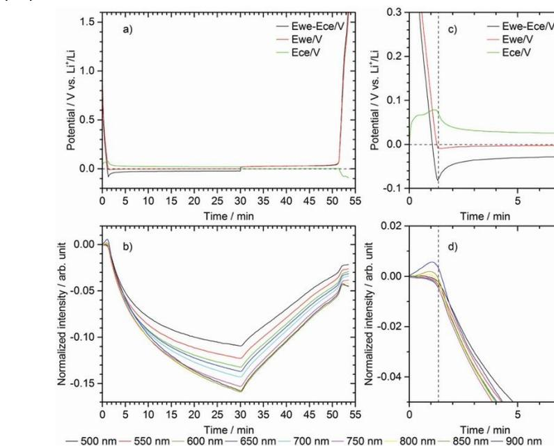
**Figure 1:** Potential profile of lithium plating and stripping in a Cu (WE) and Li (CE) half-cell (a) and corresponding intensity of the optical signal (b). The zoomed-in figures (c) and (d) present Li plating.
