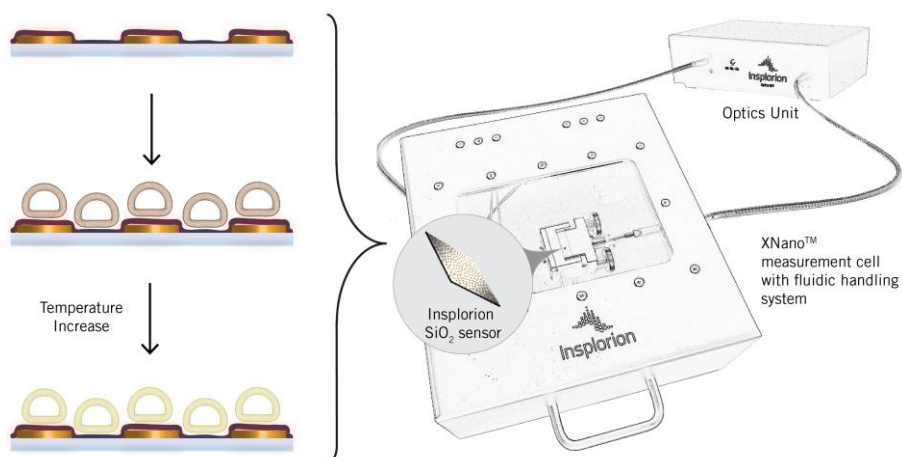
Figure 1: Insplorion system setup. The inset shows a schematic illustration of the sensors used in this application example (not to scale).
