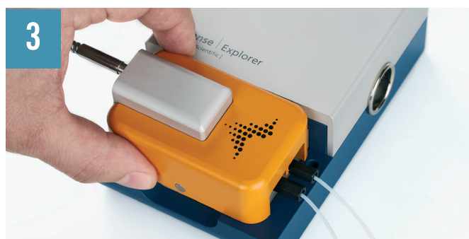
3 Connect fluidics and attach the Acoulyte module.
