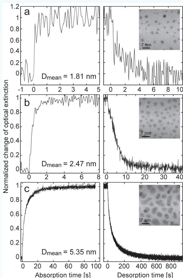
**Figure 2:** Experimental hydriding (left column) and dehydrating (right column) kinetic curves for three Pd particle diameters:  $D_{\text{mean}} = 1.81$  (a), 2.47 (b), and 5.35 nm (c). The change of the optical extinction, measured at 640 nm, is normalized that "1" corresponds to 100% conversion of the Pd nanoparticles to the hydride phase.
