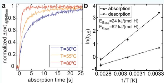
**Figure 3:** Kinetics of hydrogen storage in small Pd nanoparticles. (a) Normalized kinetic curves for hydrogen sorption in Pd nanoparticles with a mean diameter of 5.35 nm at 30, 55, and  $80^\circ\text{C}$ . The normalized optical signal is proportional to the amount of hydrogen in the nanoparticle (1 corresponds to the fully hydride state). (b) Arrhenius plots yielding activation energies of the rate limiting steps for absorption and desorption.
