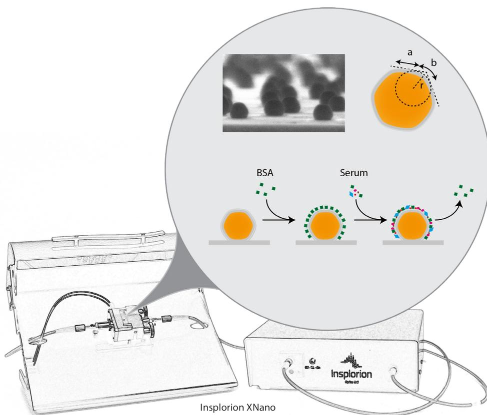
**Figure 1:** Insplorion XNano system. The ratio  $a/b$  varies with particle size while the curvature,  $r$ , remains largely constant. Biocorona formation and evolution can be followed *in situ* and in real-time.
